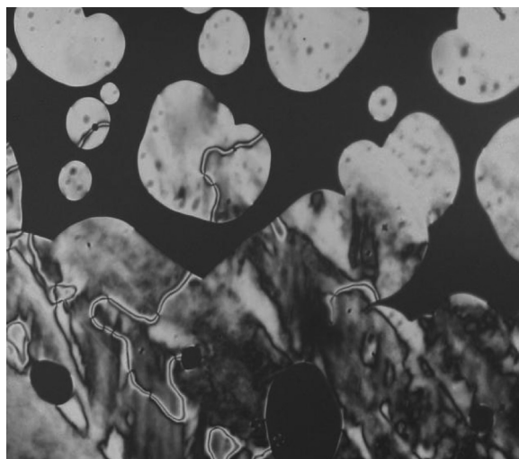
Figure 5. Texture of cholesteric phase in E_0 phase of LTA + 8BA. Texture was digitally recorded with a magnification of 10\times .
