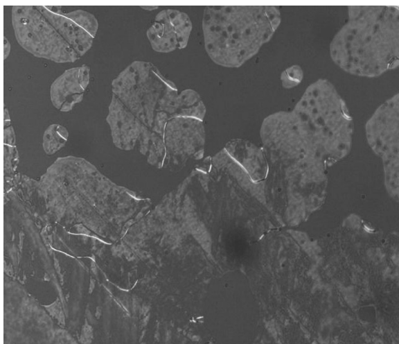
Figure 8. Texture of cholesteric phase in E_2 phase of LTA+8BA. Texture was digitally recorded with a magnification of 10\times .
